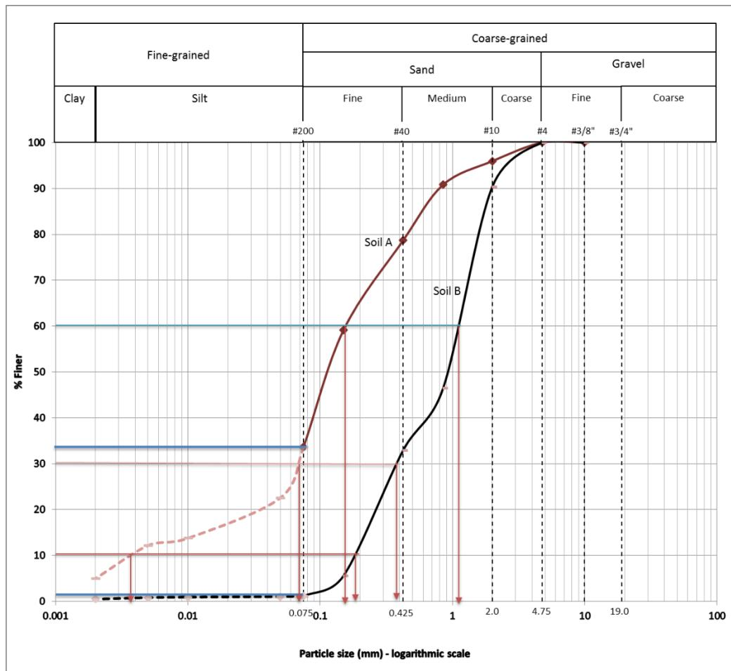
Soil A: Clay: (clay + silt + 33.7%); ; 5 % <0.002 mm; Clay = 5%, 28.7% silt
