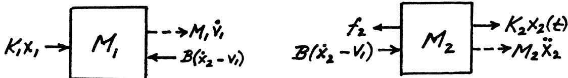
Because the motion of  $M_2$  is known, we need only the free-body diagram for  $M_1$  in order to find the state-variable equations. Summing the forces shown on that diagram, where  $\dot{x}_1 = v_1$ , we have
