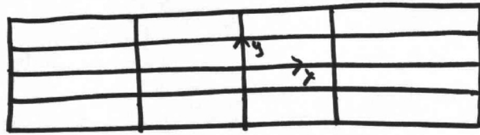
Figure 1.32: Deformation of a grid by a stagnation flow, \psi = Axy . In general, grid spacing will be closer near origin and larger far from origin; this is not terribly clear from the sketch.
