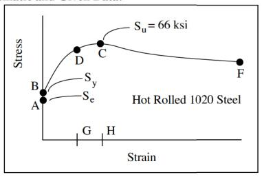
**Assumption:** After cold working the stress-strain curve for the critical location starts at point G.
