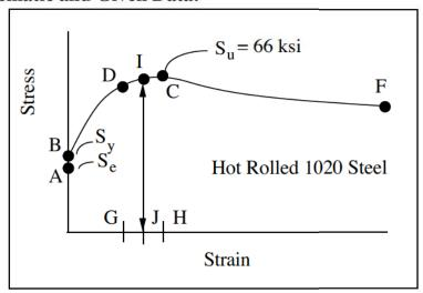
**Assumption:** After cold working the stress-strain curve for the critical location starts at point J.
