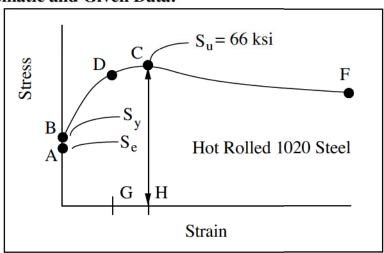
**Assumption:** After unloading the stress-strain curve starts at point H for the new specimen.
