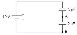
(a) How much charge does the battery deliver? You can get started by figuring out the relationship between the charges in each capacitor and the voltage across each of them.
