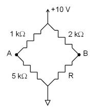
Solution: The ratio of the resistance on the two branches must be the same:
