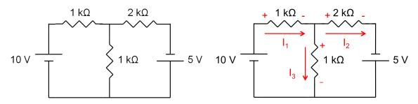
Solution: Let us assume that the currents are given in mA, resistances in k $\Omega$ and voltages in V. The equations for the left-hand and right-hand loops are:  $10-I_1-I_3 = 0$  and  $5-I_3-2I_2 = 0$ . The equation for the currents is  $I_1 = I_2+I_3$ . Solving the system of equations, we get  $I_1 = 7$  mA,  $I_2 = 4$  mA and  $I_3 = 3$  mA. The voltage drops across the middle resistor is  $(1k\Omega)(3mA) = 3$  V.
