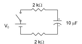
Solution: The time constant for discharging the capacitor is
