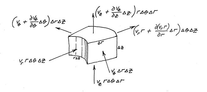
The term  $\partial M_{cv}/\partial t$  is zero because  $\rho$  is constant. Note also that the "in" arrows cancel, respectively, the leading terms of the "out" arrows. Dividing the three surviving terms by the control volume  $r\Delta\theta\Delta r\Delta z$ , we are left with
