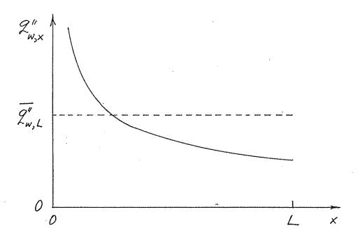
b) The relationship between the local heat flux in the middle and the L-averaged flux is obtained by first writing
