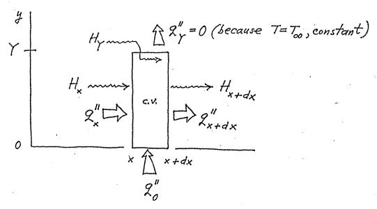
In the steady-state, the first law of thermodynamics for the control volume (c.v.) is
