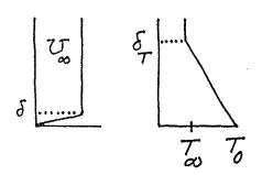
$$\frac{d}{dx} \int_0^{\delta_T} U_{\infty} \left( T_{\infty} - T_0 \right) \left( 1 - \frac{y}{\delta_T} \right) dy = \alpha \frac{T_{\infty} - T_0}{\delta_T}$$
