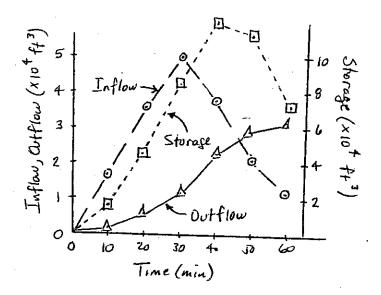
The storage increases as long as the inflow is greater than the outflow. Maximum storage occurs just prior to the point in time when outflow exceeds inflow.
