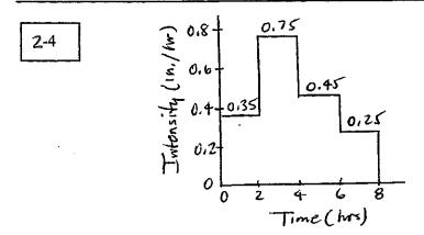
To convert the depths to intensities, divide the depths by the time interval; for example, 0.7 in./2 hr. = 0.35 in./hr.
