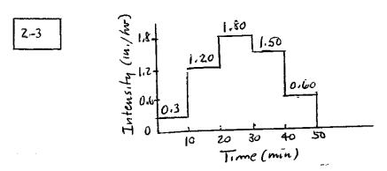
To convert the depths to intensities, divide by the interval and include conversion factors; for example, (0.05 in./10 min.) \* (60 min./hr.) = 0.30 in./hr.
