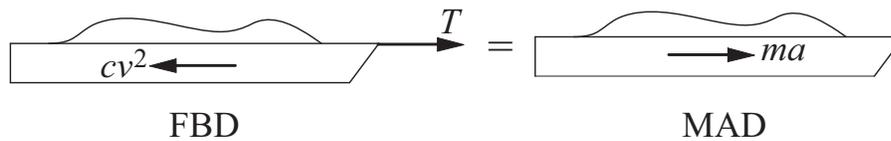
$$ma = T - F_D = T - cv^2 \quad a = \frac{T - cv^2}{m}$$
