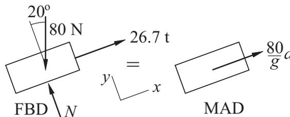
$$\Sigma F_x = ma \quad 26.7t - 80 \sin 20^\circ = \frac{80}{9.81}a$$
