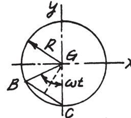
$$(b) \quad a_x = \ddot{x} = R\omega^2 \sin \omega t \quad a_y = \ddot{y} = R\omega^2 \cos \omega t$$
