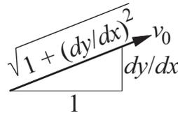
$$v_x = v_0 \frac{1}{\sqrt{1 + (dy/dx)^2}} = \frac{v_0}{\sqrt{1 + (x/500)^2}} = \frac{500v_0}{\sqrt{500^2 + x^2}}$$
