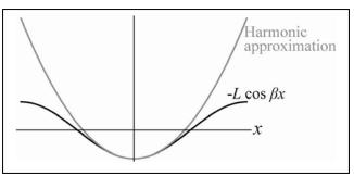
corresponds to a <u>decrease</u> in the restoring force as we go to higher amplitudes, rather than the <u>increase</u> that is required to maintain constant period. Therefore, the period increases at higher amplitudes.
