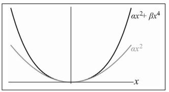
than the harmonic approximation  $U \cong \alpha x^2$ , as shown here. Since F = -dU/dx, the steeper slope corresponds to a stronger restoring force than what is required to keep the period constant. Therefore, the angular frequency increases at large amplitudes.
