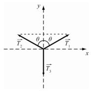
The horizontal components of  $T_1$  and  $T_2$  cancel out, so the sum  $T_1 + T_2$  is a vertical vector whose magnitude is  $T\cos\theta + T\cos\theta = 2T\cos\theta$ . The vector sum  $T_1 + T_2 + T_3$  is zero if
