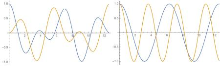
The wiggling motion is a superposition of different eigenfrequencies, but the sum and difference show the individual isolated eigenfrequencies.
