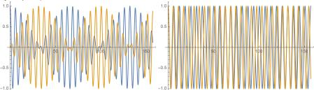
The right plot shows that the eigenfrequencies are very close to each other, resulting in the beat pattern shown in the left plot. With  $\alpha^2 \ll \omega_0^2$ , and the trigonometric identities
