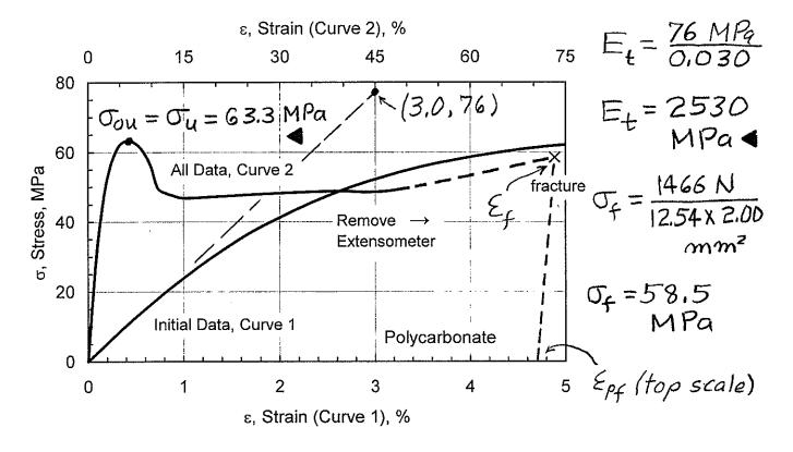
$$\begin{split} \mathcal{E}_{pf} &= \frac{\Delta L_f}{L_i} = \frac{(85.5 - 50) \, mm}{50 \, mm} = 0.71, \, 100 \, \mathcal{E}_{pf} = 71\% \, \blacktriangleleft \\ &= 100 \, \mathcal{E}_{pf} = \frac{\Delta L_f}{50 \, mm} = 0.71, \, 100 \, \mathcal{E}_{pf} = 71\% \, \blacktriangleleft \\ &= 100 \, \mathcal{E}_{f} \approx 1000 \, \mathcal{E}_{f} \approx 1000 \, \mathcal{E}_{f} \approx 1000 \, \mathcal{E}_{f} \approx 1000 \, \mathcal{E$$
