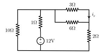
**Solution:** First we label the nodes from 1 to 3. While a node number can be given to any intersection of multiple wires, we can assign 1 at two intersection points with a direct connection between them.
