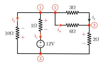
We also define the current directions (completely arbitrarily) and potentials across the components accordingly using the sign convention. Note that, following the sign convention, the current across a component flows from its positive terminal to negative terminal. Now, we can apply KVL and KCL to solve the problem. First, consider the loop from node 1 to node 2 and back to node 1. We have
