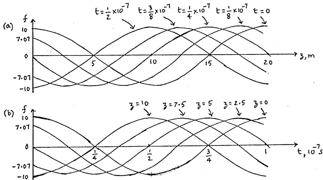
$f(z, t)$  represents a traveling wave progressing with time in the negative  $z$ -direction.
