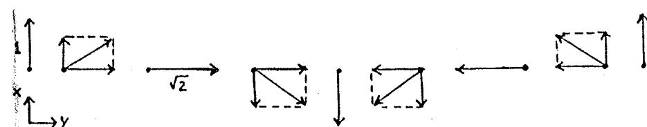
The polarization is elliptical with major axis in the  $y$ -direction, minor axis in the  $x$ -direction, and eccentricity equal to  $\sqrt{2}$ .
