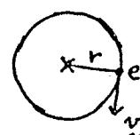
$$\text{Orbital frequency} = \frac{\omega}{2\pi} = \frac{eB_0}{2\pi m}$$
