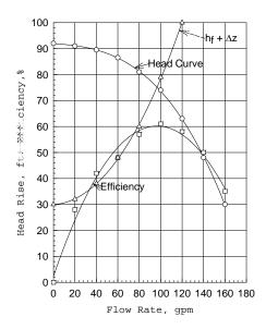
frictional resistance as  $h_f=f(L/D)(V^2/2g)=0.00459 \text{ Q}^2\text{gpm}$ . In this problem, we must add  $\Delta z$  to  $h_f$  to equate to  $H_{pump}$ . The solution then becomes  $H_{pump}=0.00459 \text{ Q}^2+30$ . On the graph at right, the solution is Q=100 gpm at H=74 ft and  $\eta=0.60$  (i.e., the BEP).
