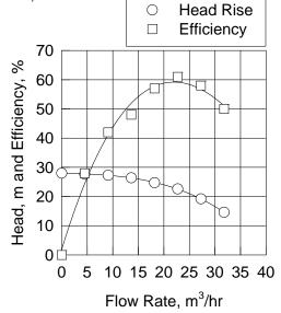
Solution: In Problem 1.15 we developed the H-Q curve in  $m^3/hr$  and m of head. We show these curves here for reference. The only difference here is the coefficient of resistance for the system. Here Kres =  $f(L/D) + \sum K_m = f(L/D) = 0.030(100/.05) = 60$ . The h<sub>f</sub> curve becomes  $0.0612Q^2$  with Q in m<sup>3</sup>/hr. The intersect with the pump curve is atapproximately  $Q=19.5 \text{ m}^{3}/\text{hr}$  at 23.6 m of head.
