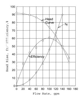
Re<sub>D</sub> (i.e., >4x10<sup>5</sup>), f=0.027. Combining the numbers yields  $h_f$ =45.8 (Q<sub>gpm</sub>/100)<sup>2</sup> in feet of head. Superposing on the pump curve shows the intersect occurring at about 118 gpm.
