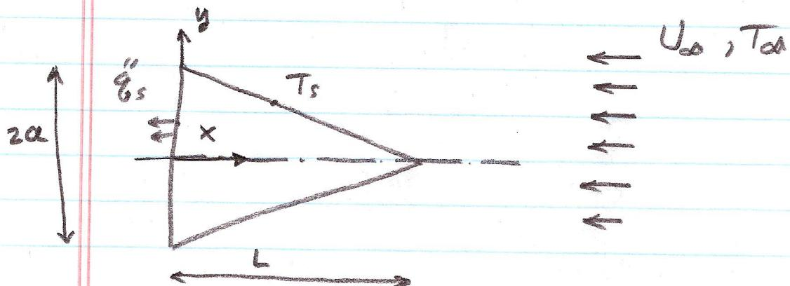
Assume the fluid is incompressible & constant-property. Also, assume that the process is steady-state, and the flow field is 2D. Without symmetry:
