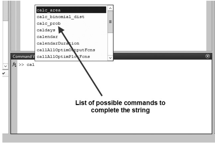
Figure 1.11 If you type a partial command and then hit the Tab key, MATLAB will pop up a window of suggested commands or functions that match the string.
