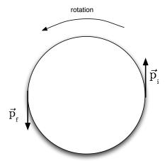
To find the change in momentum, sketch  $\vec{p}_{\rm f}$  and  $\vec{p}_{\rm i}$  tail to tail.  $\Delta \vec{p}$  is the vector from the head of  $\vec{p}_{\rm i}$  to the head of  $\vec{p}_{\rm f}$ . See the figure below..
