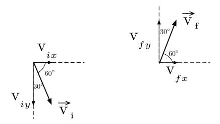
The angle of the vector with the +y axis is  $30^{\circ}$ , and the angle with the +x axis is  $60^{\circ}$ . The vector's components can be easily calculated using the cosine of each of these angles. Thus
