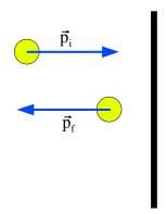
Sketch the change in momentum vector by drawing the initial and final momentum vectors tail to tail and drawing the change in momentum from the head of the initial momentum to the head of the final momentum, as shown in the figure below..
